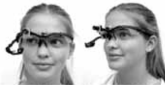
Figure 1- Lightweight, dark pupil, eyetracking headgear
