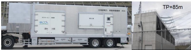
(a) 4000 kVA mobile gas-turbine generator at 31 m parking and GIS at 85 m height (Hepco).
