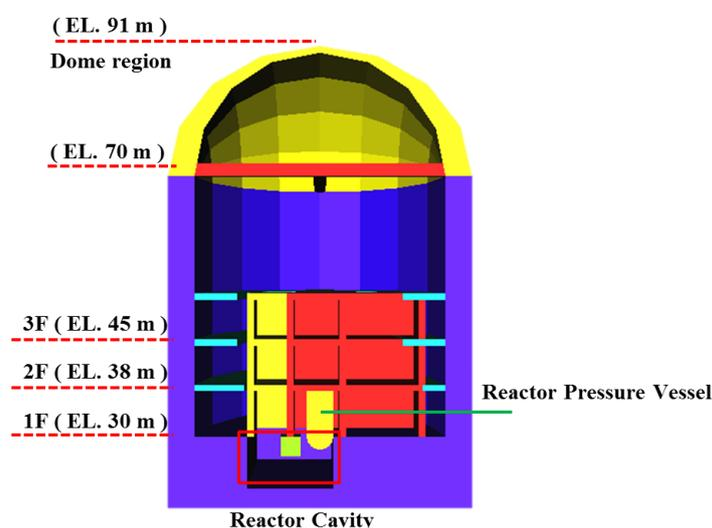
Fig. 1 Cross section of 3D reactor and containment model used in FLACS.
