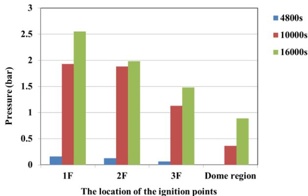
Fig. 7 Predicted pressure loads at different ignition time and points.
