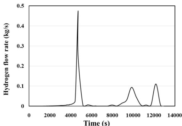
Fig. 3 The variation of the mass flow rate with time.
