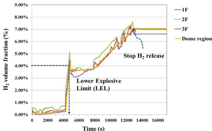
Fig. 4 Change in hydrogen volume fraction over time in containment building. Concentration sensors are located on the ground of the 1<sup>st</sup> floor (1F), 2<sup>nd</sup> floor (2F), 3<sup>rd</sup> floor (3F), and the center of the dome region (Dome region).
