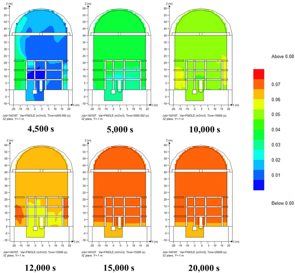
Fig. 5 2D cross section of hydrogen distribution.
