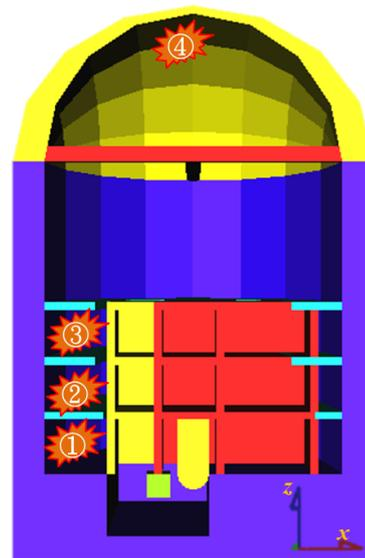
Fig. 6 The ignition points in the containment building. Points 1–3 are located on floors 1–3, respectively, and point 4 is located in the dome region.
