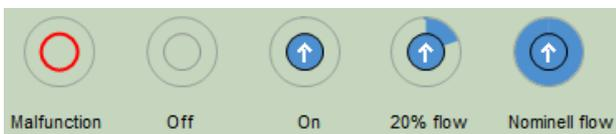
Fig. 3 Combined pump status and flow from the pump.
