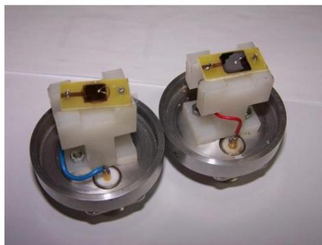
Fig.3 Current mode GaN detector.
