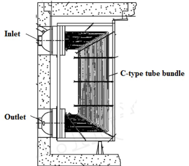
Fig.2 The passive residual heat removal heat exchanger.
