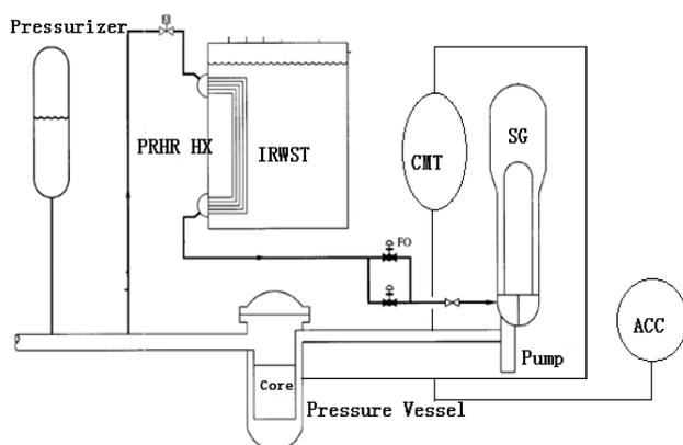
Fig.1 AP1000 main loop system and passive core cooling system.
