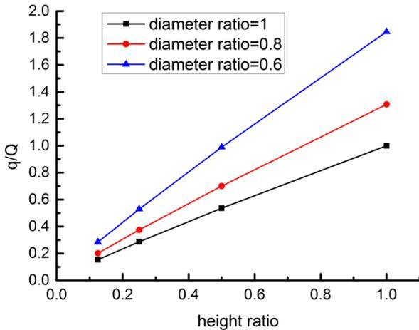
Fig.3 The ratio between heat exchange capacity and core power changes with the height ratio under different diameter ratios.
