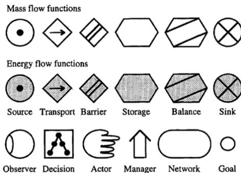
Fig.3 Symbols of multi-level flow model.
