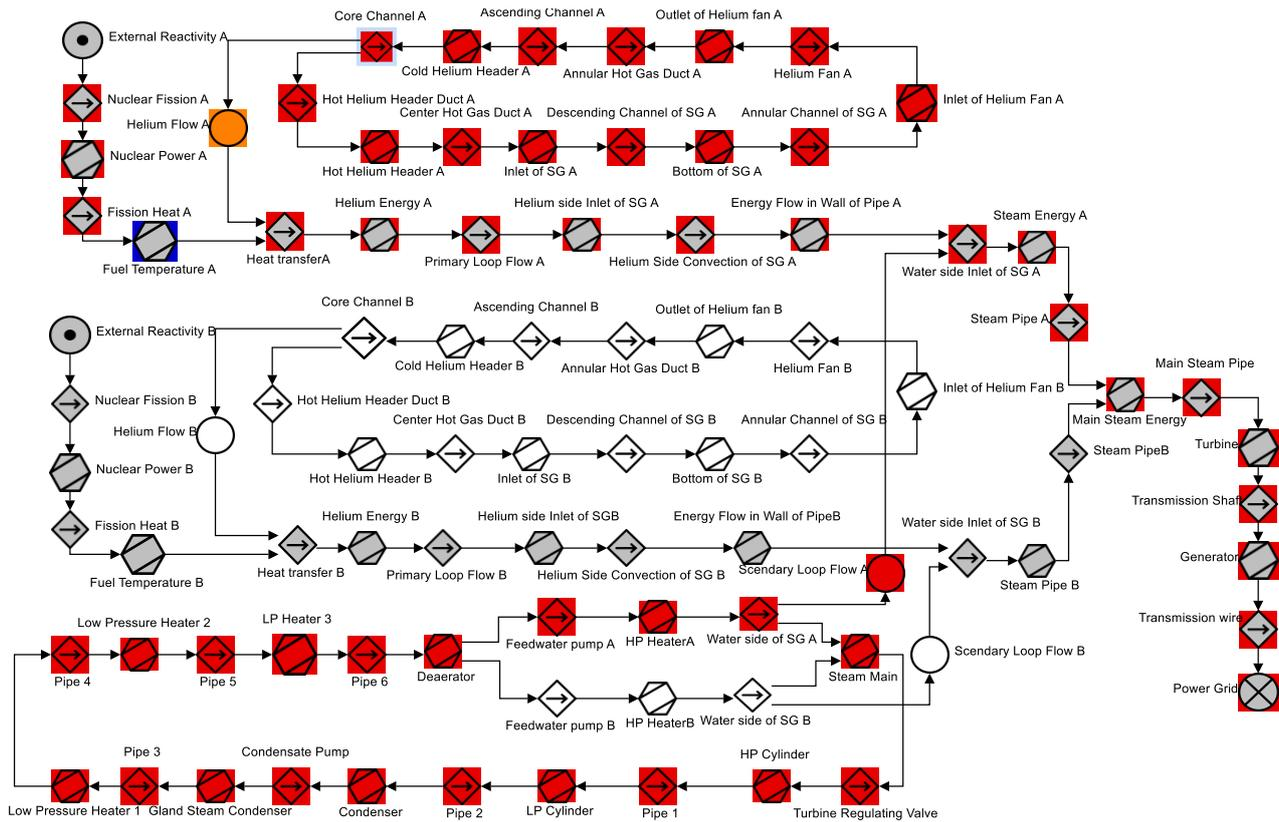
Fig.4 Fault propagation path.
