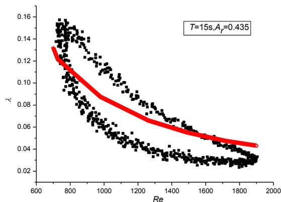
Fig. 6 Annular curve in the laminar flow.
