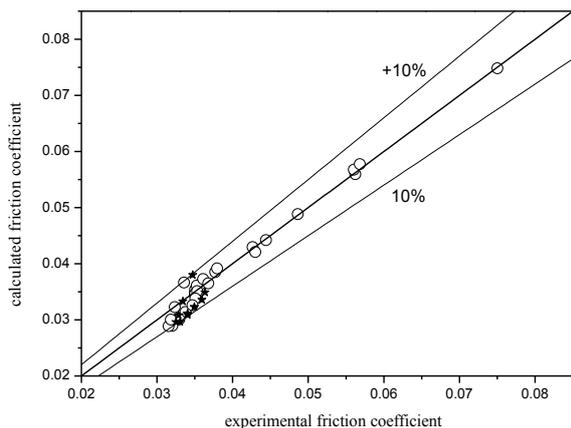
Fig. 11 Performance of the correlation for predicting the magnitude of the friction coefficient.
