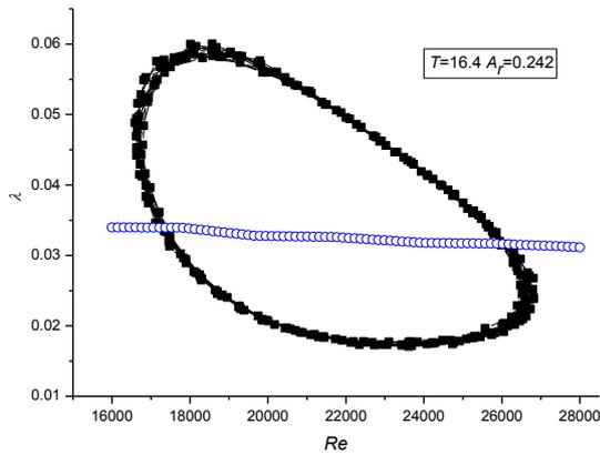
Fig. 8 The transient friction coefficient and the steady flow friction coefficient in a circular tube.
