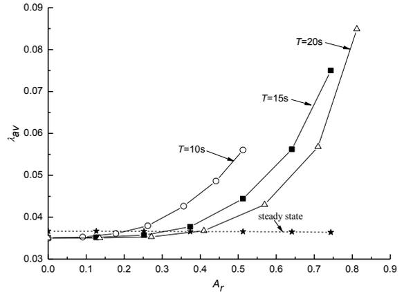
Fig. 10 Time-averaged friction coefficient under different cases in a rectangular channel.
