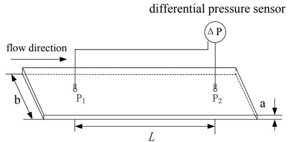
Fig. 2 Schematic of test section.
