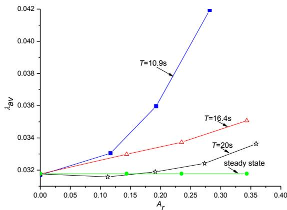
Fig. 9 Time-averaged friction coefficient under different cases in a circular tube.
