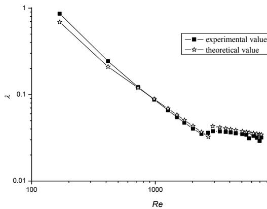
Fig. 3 Verification of experimental system with rectangular channel.
