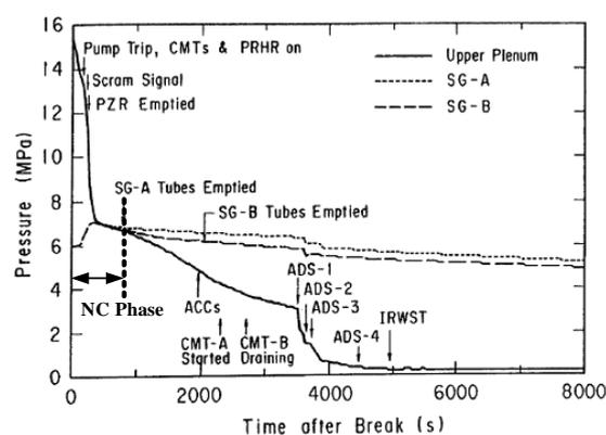
Fig.1 The pressures in primary and secondary side of SG in AP600 during a 1-in. cold leg break test on ROSA<sup>[4]</sup>.
