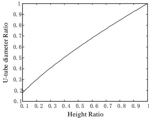
Fig.4 U-tube diameter ratio versus system height ratio.
