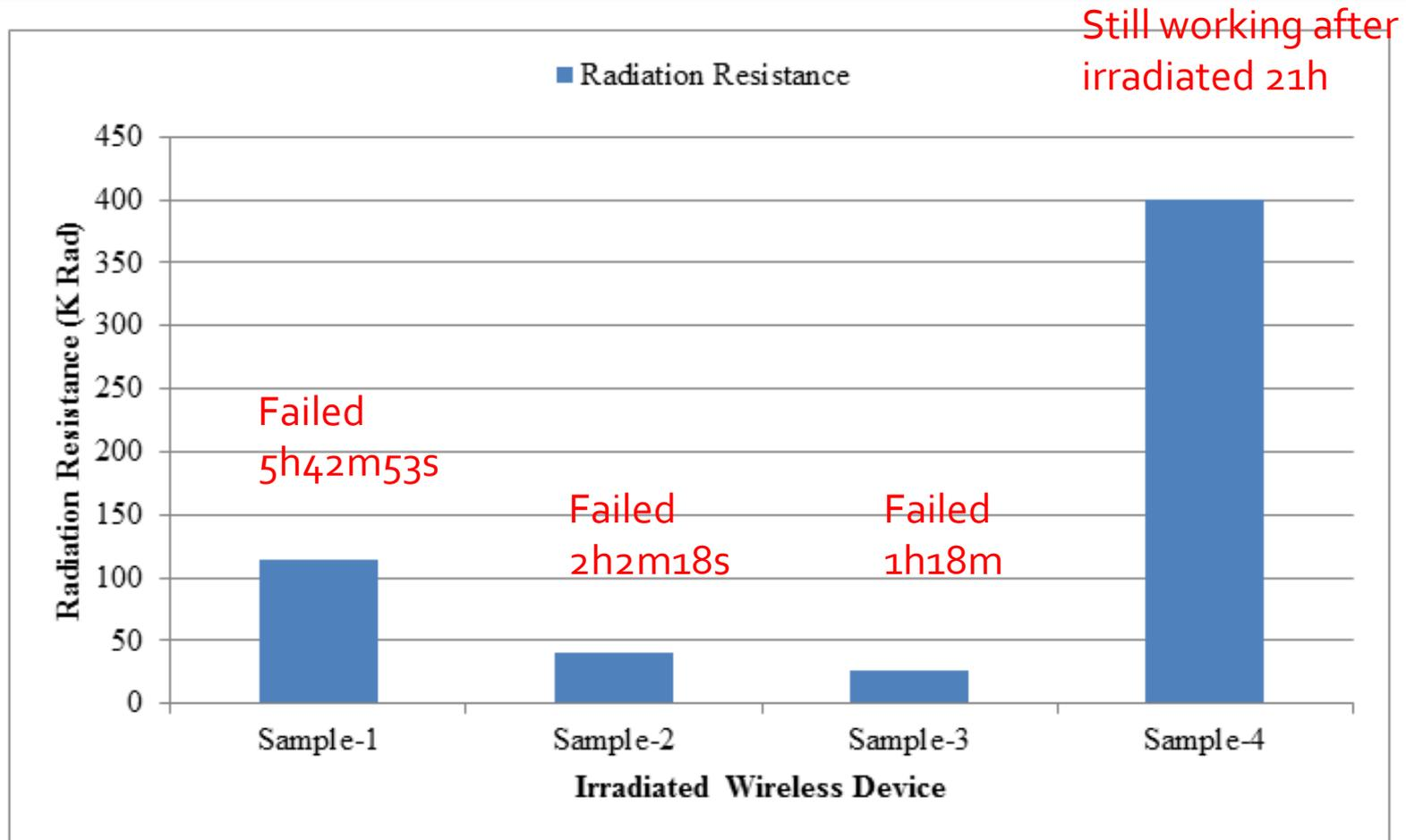
Comparison of radiation resistances of wireless devices under a high dose rate condition (20 K Rad/h)
