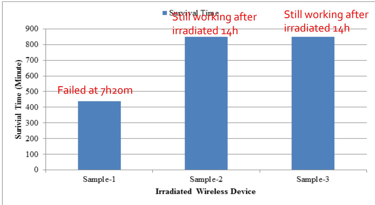
Comparison of radiation resistances of wireless devices under a low dose rate condition (200 Rad/h)
