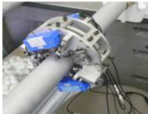
Fig. 7 Guided wave sensor.
