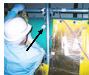
Fig. 2 Example of a CZT measurement The probe is on contact.
