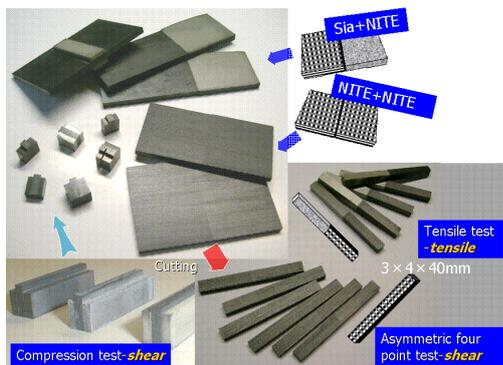
Fig. 9 NITE-SiC joints and test specimens.
