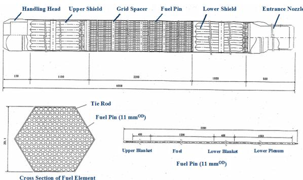
Fig. 11 GFR core design concept using fuel pin.
