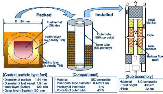
Fig. 10 FGR core and fuel concept [10].
