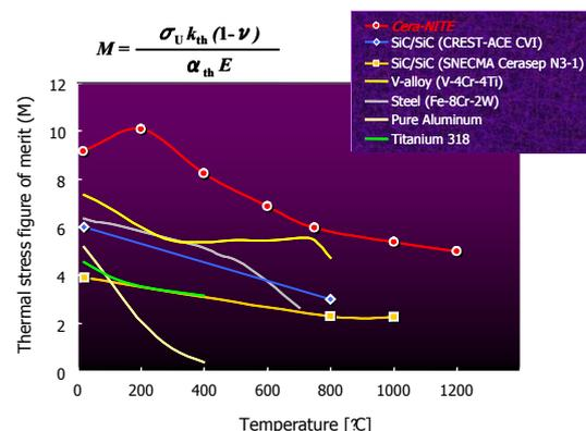
Fig. 6 Excellence in thermal stress resistance as shown by thermal stress figure of merit M.
