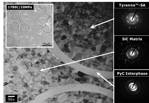
Fig. 5 Microstructure of NITE SiC/SiC.
