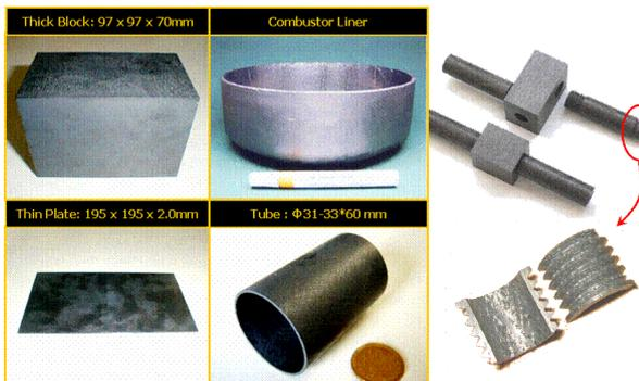
Fig. 4 Shape flexibility of NITE SiC/SiC composites.
