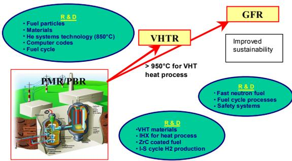
Fig. 1 Gas Reactor Technology and R & D Pathway [8].
