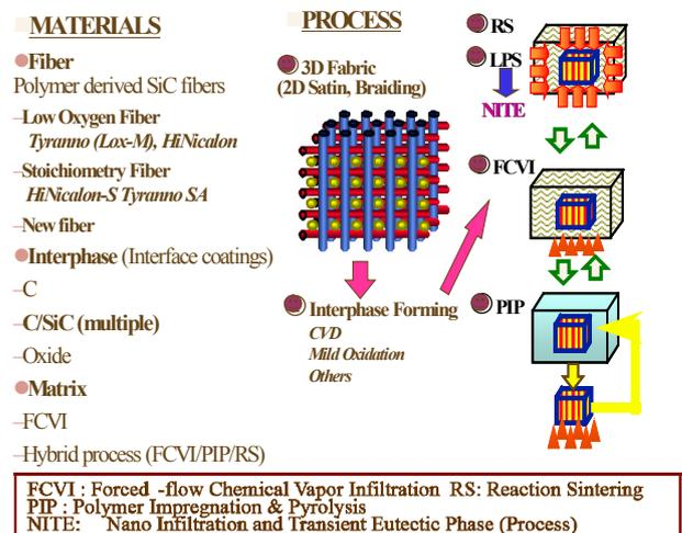
Fig.2 Ceramic matrix composite ; components and processing.
