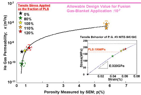
Fig. 8 Effect of deformation on He permeability.
