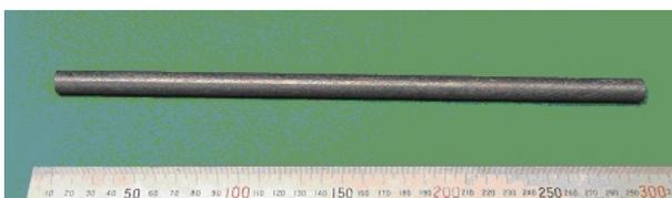
Fig. 12 2D SiC/SiC tube for GFR by NITE process.
