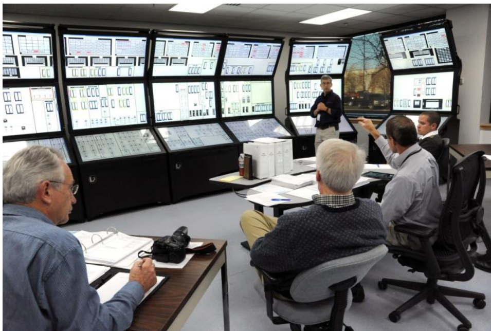
Fig. 4. HSSL being used for control room design activities with licensed operators.
