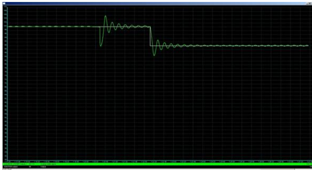
Results of control logic tuning(Filter off)
