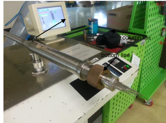
Fig.11 Helium leak test setup.
