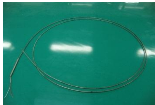
Fig.4 K-type thermocouple specimen.
