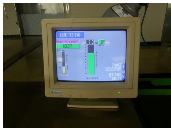
Fig.12 Seal performance test result.
