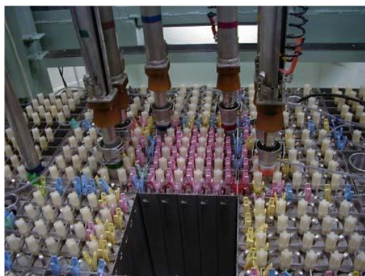
Fig. 2 Example of the KUCA Solid-Moderated Core (B-core), showing fuel elements, control rods and removable section of the core (in shutdown position).
