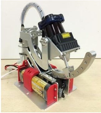
Fig.2 Real-time 3D laser scanner which we have developed.
