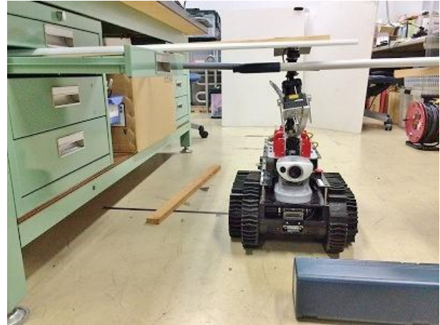
Fig.10 Experimental environment for the range of obstacle detections. There are some polls and plates over the mobile robot and a black object on the ground near the mobile robot.
