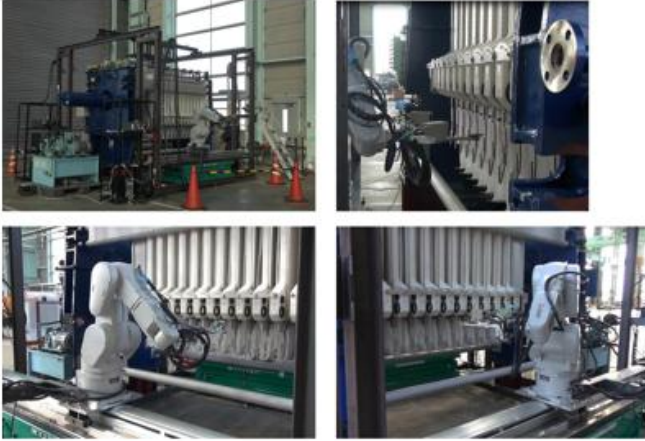
Fig. 1: Two 3D-MoS robot system with dual hand-eye cameras set beside filter press decontamination machine for full automatic exchanging of cloths of filter press.
