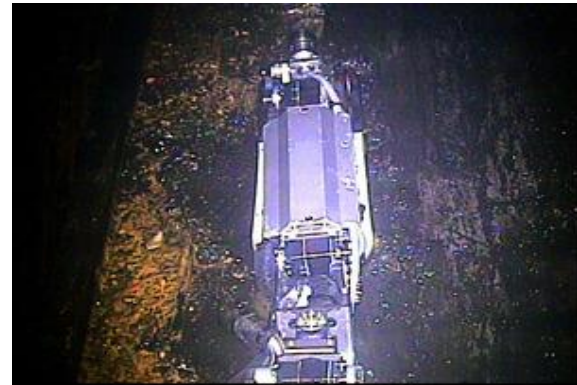
Fig. 1 The Sasori (Scorpion) robot is stuck inside the containment vessel of No. 2 reactor of Fukushima Daiichi nuclear power plant.
