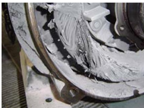
Photo 4 Interlayer short of coil winding.
