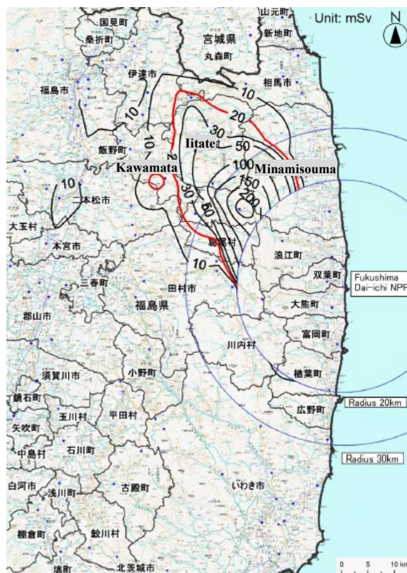
Fig.13 Estimated contour map of integrated dose (Until May 11, 2012) showing discharge of radioactive material by hydrogen explosion toward north west direction from Fukushima Daiichi NPS.
