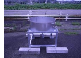
(c) Dust sampling equipments for monitoring radioactive materials were installed in plant.
