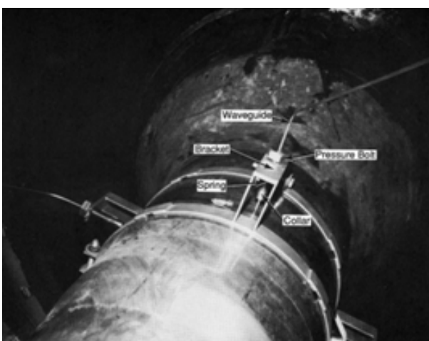
Fig. 3 AE sensor in place at Limerick NPP (NUREG/CR-5963) [2].
